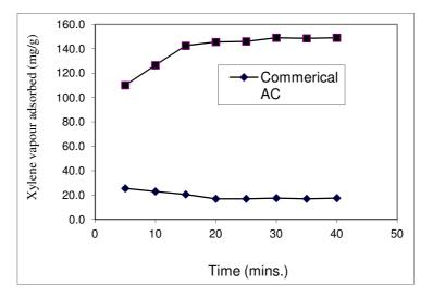
Fig. 9 Rate of Adsorptiion of Xylene vapour by commercial and bamboo activated carbon
