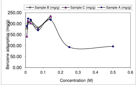
Fig 3. Effect of activation with Trioxonitrate (v) acid on benzene adsorption of activated carbon using activated carbon from Nigerian bamboo
