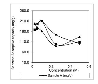
Fig. 1 Effect of activation with tetraoxosulphate (vi) acid on Benzene vapour Adsorption using activated carbon from Nigerian bamboo
