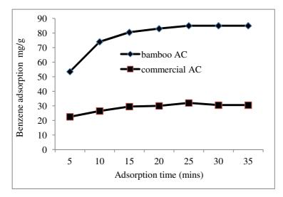
Fig. 8: Rate of Adsorptiion of benzene vapour by commercial and bamboo activated carbon
