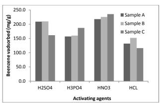
Fig 7: Shows the effect of activating agent on benzene adsorption using different Nigerian bamboos
