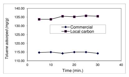
Fig. 10 Comparison of Adsorption rate of Toluene vapour using bamboo and Commercial activated carbon
