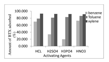
Fig 6 BTX adsorbed in aqueous solution using activated carbon from bamboo activated with different activating agent
