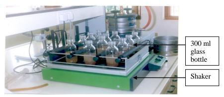
Plate1: Phosphorus sorption experiments in a slow rotating shaker
