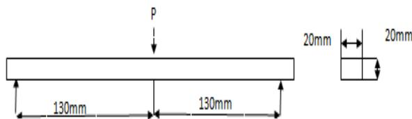
(a) Bending strength test arrangement (Central loading)
