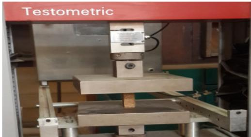
(b) Compression stress parallel to grain test set up
