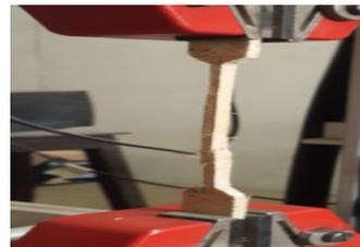
(a) Tensile test sample geometry
