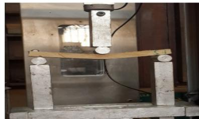
(b) Static bending failure mode
