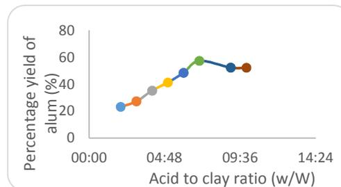
**Fig 7:** Effect of acid to solid ratio on the extraction of the alum (leaching time: 1.5 h; temperature: 110°C; particle size: 100 $\mu\text{m}$ ; acid concentration: 5M)
