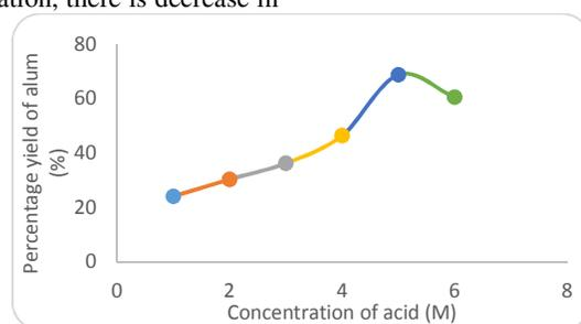
**Fig 8:** Effect of H<sub>2</sub>SO<sub>4</sub> concentration on the extraction of alum (leaching time:1.5 h; temperature:110°C; particle size: 100 μm)
