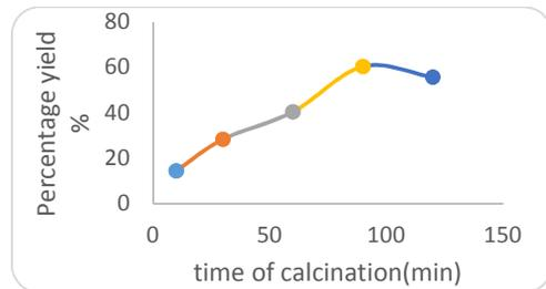
**Fig 3:** Effect of calcinations time on the extraction of alum (particle size: 100  $\mu\text{m}$ , temperature: 800°C).
