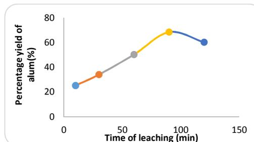
**Fig 6:** Effect of leaching time on the extraction of alum (acid concentration: 5M; particle size: 100  $\mu\text{m}$ ; temperature: 110°C)
