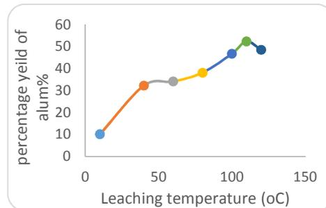
**Fig 5:** Effect of leaching temperature on the extraction of the alum (leaching time: 1.5 h; acid concentration: 4M; particle size: 100  $\mu\text{m}$ .)
