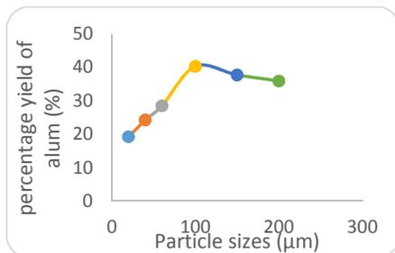
**Fig 4:** Effect of particle size on the extraction of alum (leaching time: 1.5 h, temperature: 80°C; acid concentration: 4M).
