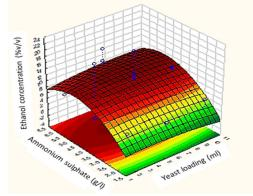
Fig 3: 3D response plot showing the effect of yeast loading and ammonium sulphate on ethanol production
