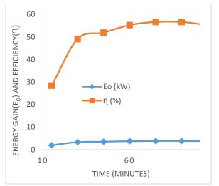
Fig 3: The Variation of Time with Energy Gain and efficiency of the Sawdust Oven
