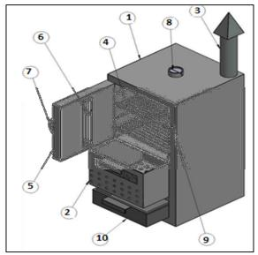
**Fig 1**: Isometric view of Sawdust Fired Oven: *Parts: 1 = frame; 2 = burner; 3 = chimney; 4 = shelves; 5 = door; 6 = transparent glass; 7 = handle; 8 = flap; 9 = insulation; 10 = ash tray*
