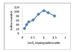
Fig 1: Variation of ZnCl2 impregnation ratio with iodine number
