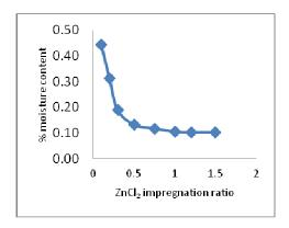
Fig 6: Effect of ZnCl2 impregnation ratio on moisture content of
