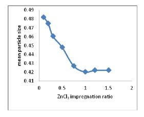
Fig 9: Effect of ZnCl<sub>2</sub> impregnation ratio on mean particle size of PSC
