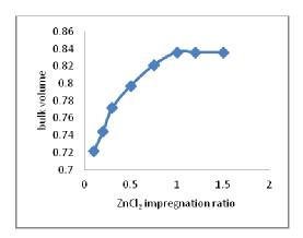
$\textbf{Fig 8:} \ Effect \ of \ ZnCl_2 \ impregnation \ ratio \ on \ bulk \ volume \ of \ PSC$
