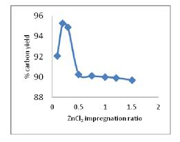
Fig 5: Effect of ZnCl<sub>2</sub> impregnation ratio on carbon yield of PSC
