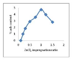
Fig 2: Effect of ZnCl<sub>2</sub> impregnation ratio on ash content of PSC
