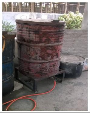
Plate 1: Fabricated Wet Steam Sterilizing Unit. UNIPORT Mushroom Unit
