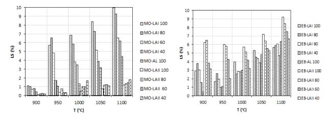
Fig. 5. Linear shrinkage variation with firing temperature of Monatele and Ebebda tested bricks
