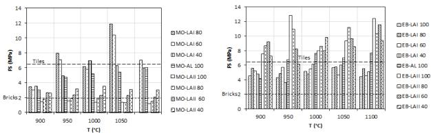
Fig. 7. Flexural strength variation with firing temperature of Monatele and Ebebda tested bricks
