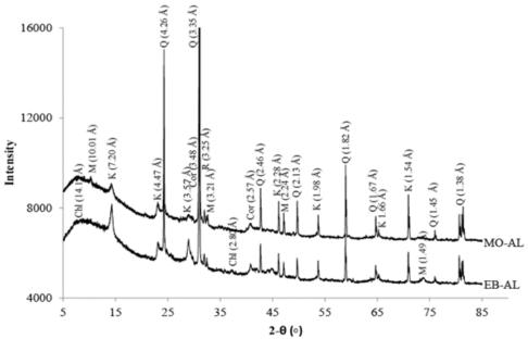
Fig. 2. X-ray diffraction pattern of the alluvial clays of Monatele and Ebebda
