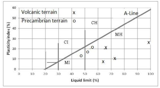
Fig. 4: Classification of Samples using the Plasticity Chart (after Casagrande)
