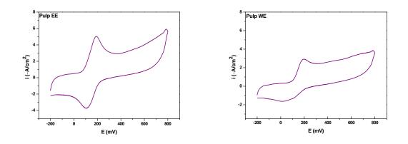
**Fig.4.** Cyclic voltammograms of **pulp** of **dark purple eggplant** EE and WE extracts in pH 7, 0.2M phosphate buffer solution at scan rate 100 mV/s.
