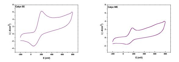
**Fig.5.** Cyclic voltammograms of **calyx** of **dark purple eggplant** EE and WE extracts in pH 7, 0.2M phosphate buffer solution at scan rate 100 mV/s.
