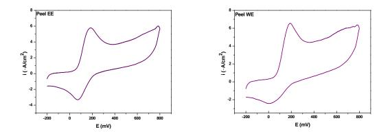
**Fig.3.** Cyclic voltammograms of **peel** of **dark purple eggplant** EE and WE extracts in pH 7, 0.2M phosphate buffer solution at scan rate 100 mV/s.
