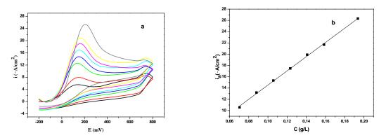
Fig.2. Cyclic voltammograms referring to different ascorbic acid concentrations (a), calibration curve obtained by cyclic voltammetry method expressed as ascorbic acid equivalents/L (b).
