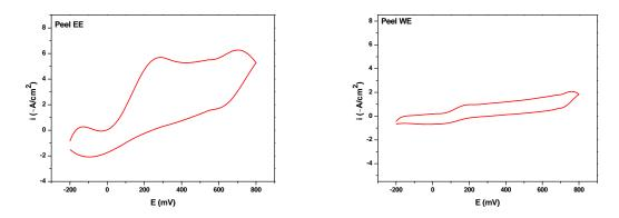
**Fig.6.** Cyclic voltammograms of **peel** of **white eggplant** EE and WE extracts in pH 7, 0.2M phosphate buffer solution at scan rate 100 mV/s.
