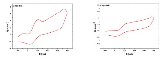
**Fig.8.** Cyclic voltammograms of **calyx** of **white eggplant** EE and WE extracts in pH 7, 0.2M phosphate buffer solution at scan rate 100 mV/s.
