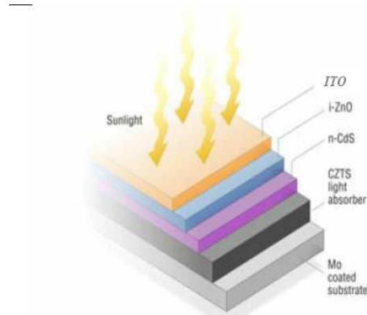
**Fig.1.** Structure of a photovoltaic cell CZTS
