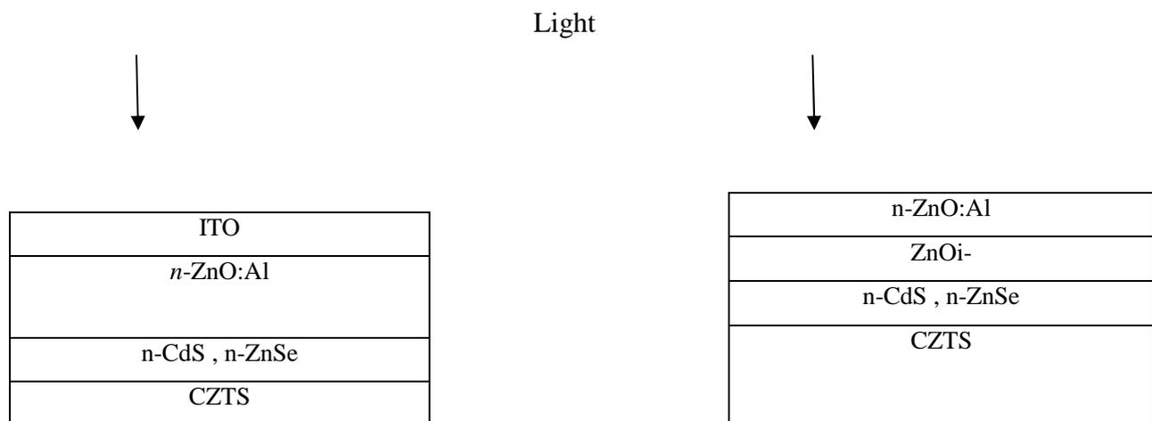
**Fig.2.** Structure of Solar cell
