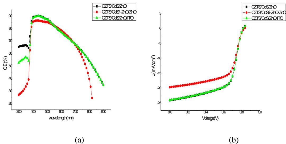
**Fig.3.** a) Characteristic I-V of the first configuration of the CZTS cell, b) the spectral response with the CdS buffer layer
