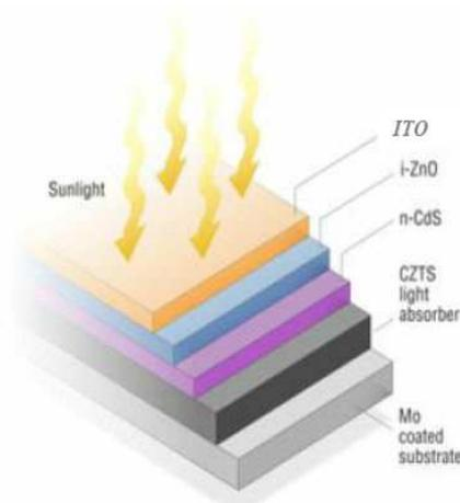
**Fig.1.** Structure of a photovoltaic cell CZTS
