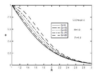
**Fig.3.** Effect of Grashof number (Gr) on dimensionless temperature Profiles for  $\chi = 0$  and time-dependent axial velocity of cylinder  $U(\ddagger) = \exp(-\ddagger)$
