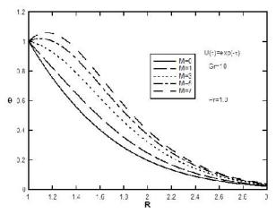
Fig.5. Effect of magnetic parameter (M) on dimensionless temperature Profiles for x = 0 and time dependent axial velocity of cylinder  $U(\ddagger) = \exp(-\ddagger)$
