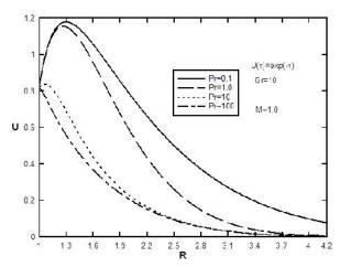
Fig.6. Effect of Prandtl number on dimensionless velocity
