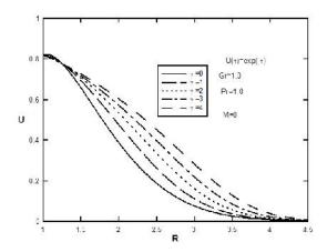
Fig.8. Effect of viscosity-variation parameter (x) on dimensionless velocity
