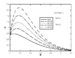
**Fig.2.** Effect of Grashof number (Gr) on dimensionless velocity Profiles for x = 0 and time-dependent axial velocity of cylinder  $U(\ddagger) = \exp(-\ddagger)$
