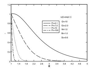
Fig.7. Effect of Prandtl number on dimensionless temperature
