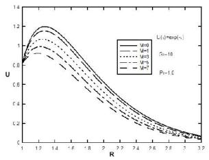
Fig.4. Effect of magnetic parameter (M) on dimensionless velocity
