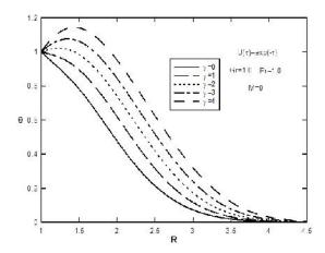
**Fig.9.** Effect of viscosity-variation parameter ( $\chi$ ) on dimensionless temperature
