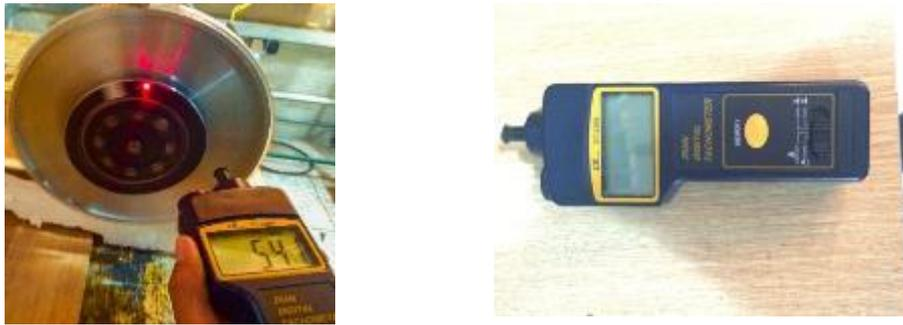
**Fig. 8.** Inverter device and laser tachometer, to adjust the engine speed is used. A reflecting laser tag located on the flywheel. Inverter on the one hand input of the engine and on the other to the three-phase is connected. The relationship Between the Frequency inverter and motor to a linear relationship. The test started of 30 RPM to 400 RPM and calculated. As you can see around 400 RPM equivalent to 20 Hz.
