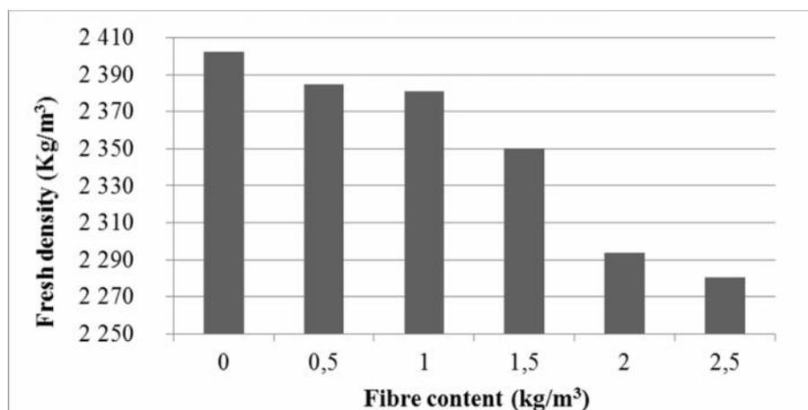
**Fig.2.** Variation of the density in a fresh state of the various types of RCC
