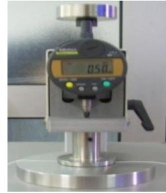
**Fig.3.** Thickness gauge
