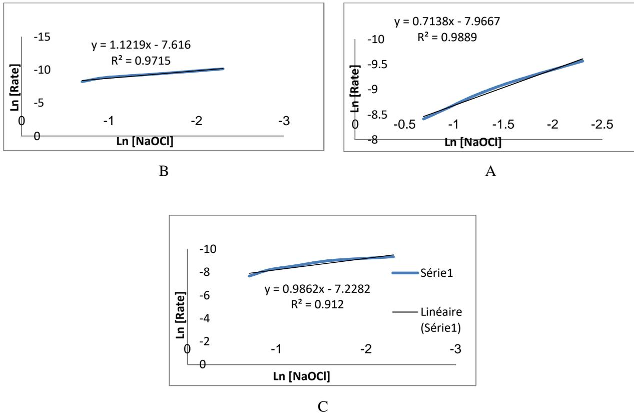
**Fig.2.** Plot of  $\text{Ln}[\text{Rate}_2]$  in terms of  $\text{Ln}[\text{NaClO}]$  at three temperatures: A: fridge (4 °C), B: room temperature (20 °C) and C: oven temperature (47 °C)
