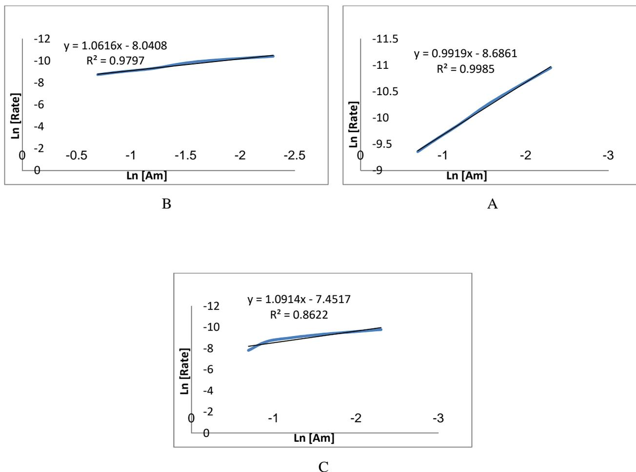
**Fig.3.** Plot of  $\text{LnRate}_3$  in terms of  $\text{Ln}[Am]$  at three temperatures: A: fridge (4 °C), B: room temperature (20 °C) and C: oven temperature (47 °C)
