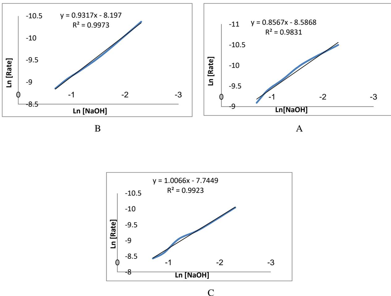
**Fig.1.** Plot Ln[Rate] in terms of Ln[NaOH] at three temperatures: A: fridge (4 °C), B: room temperature (20 °C) and C: oven temperature (47 °C)
