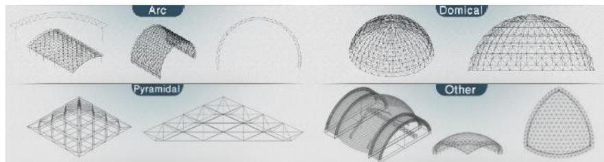
Figure 6.3. 3D truss Qvsaydownload: Chyltvn2009
