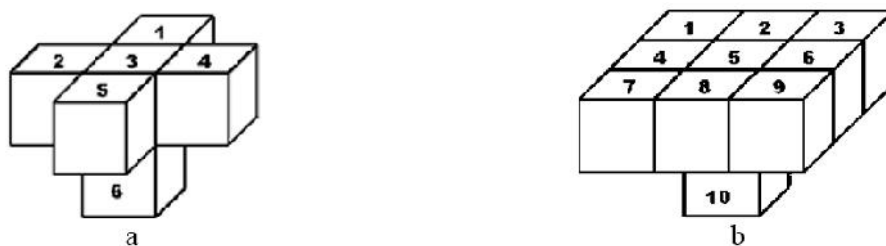
Fig.2. Sequencing rules can be based, for example, on the removal of five blocks above a given block, block 6 (a) or on the removal of nine blocks above a given block, block 10 (b).
