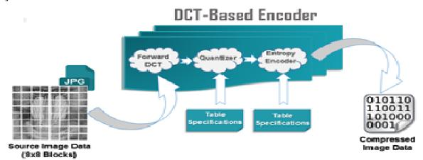
Fig.5. A DCT-Based encoder model
