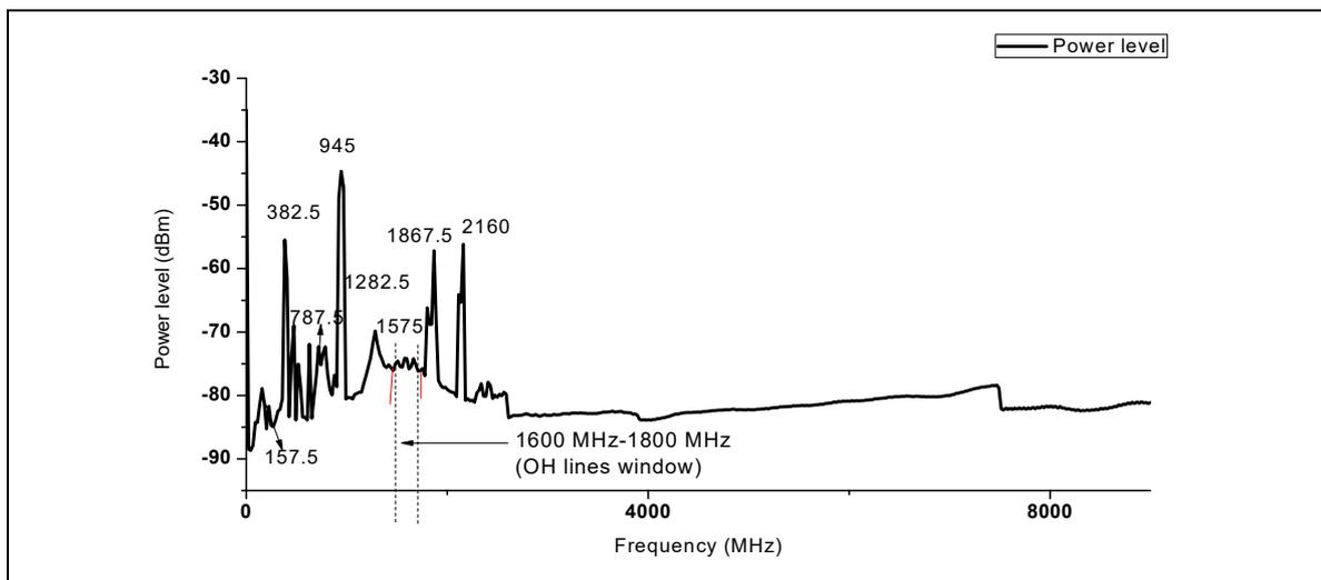
**Fig.1.** RFI spectrum in wide window (0-9000MHz)
