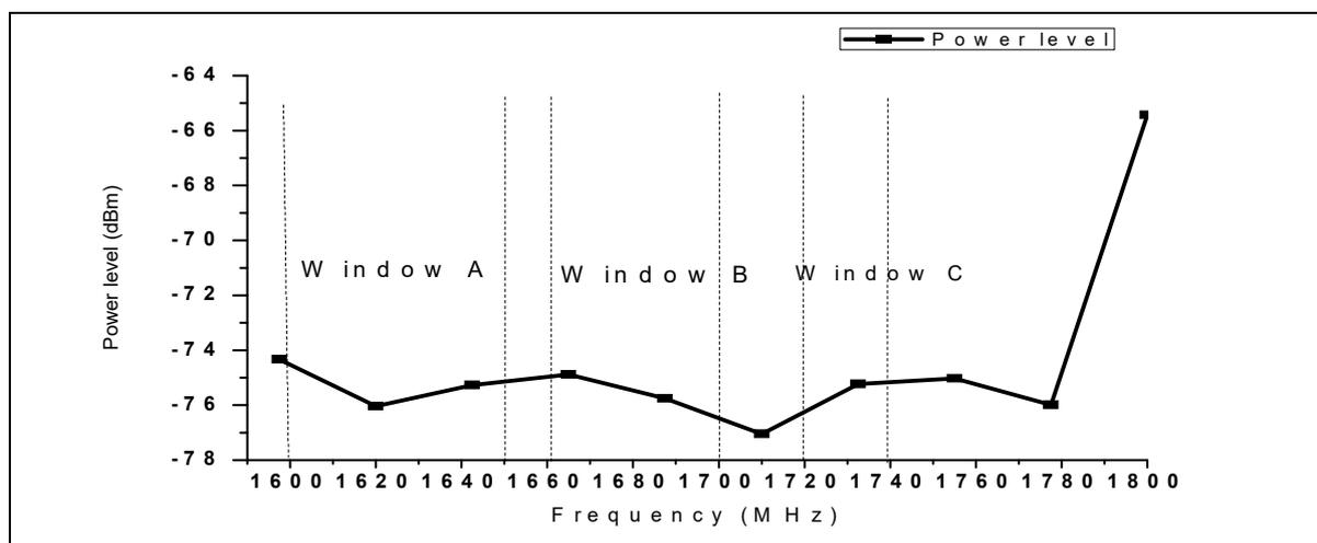
**Fig.2.** RFI spectrum in OH lines window (1600MHz-1800MHz)
