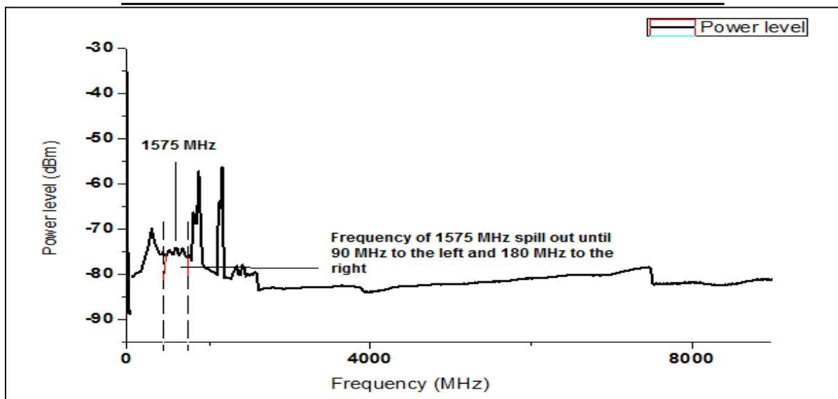
**Fig.3.** Frequency of 1575 MHz spill out from their frequency until take part in OH lines window
