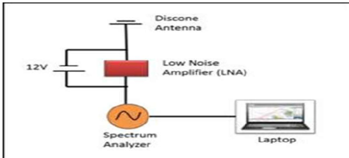
**Fig.4.** Instrument setup for RFI observation [15]
