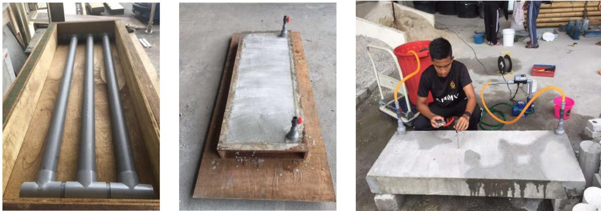
a) PVC pipes inside the panel      b) Casted slab panel      c) Tested of temperature of slab with water flowing inside the panel
