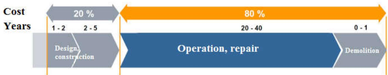
**Fig.1.1.** Cost relationship on different stages of a heat supply facility life cycle
