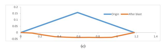
Fig.5. Deformation of the V plate after explosion (a) V plate 90° (b) V plate with 120° and (c) angle 150° of plate
