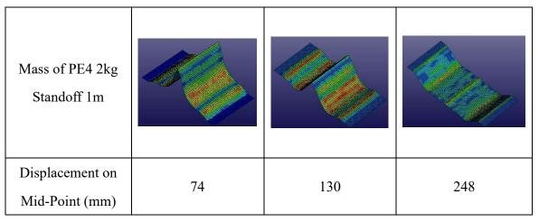
Fig.3. Contours of displacement between Plastic Kinematic model and Johnson Cook model
