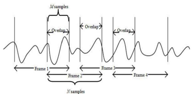
Fig.8. Illustration of framing process
