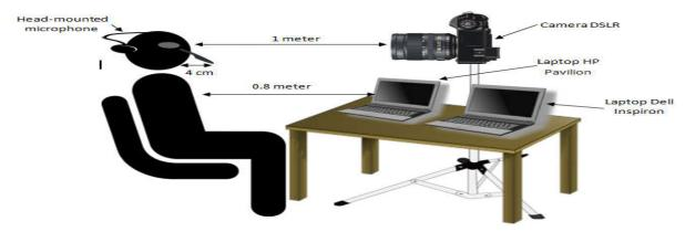
Fig.3. The recording setup
