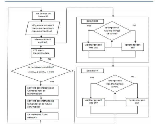
Fig.8. Flowchart of capacity based handover scheme
