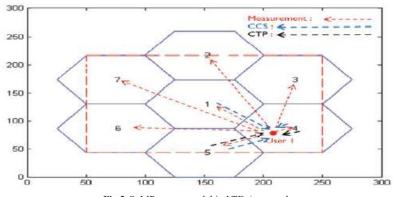
Fig.2.CoMPsystem model in LTE-A network
