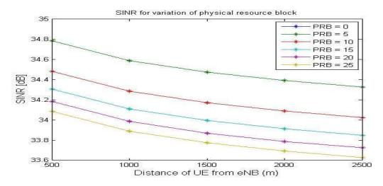
Fig.4. SINR versus distance of UE from BS with variation of PRB
