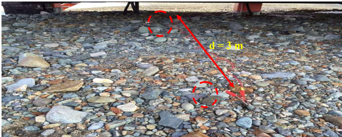
Fig.5. Electrodes are placed into the ground which are connected to the resistivity meter using cables
