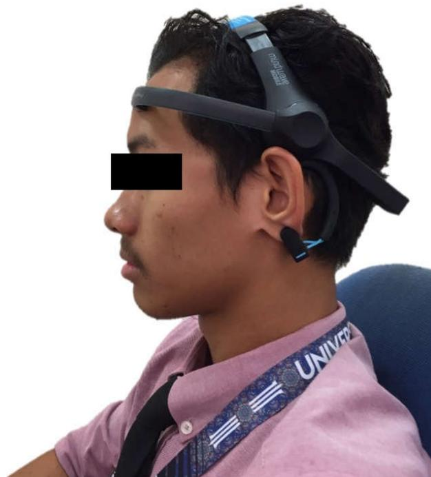
**Fig.2.** Placement of Neurosky Mobile Wave headset
