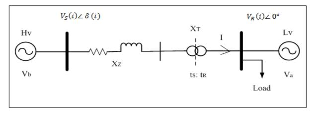
Fig.1. Electric equivalent of system network
