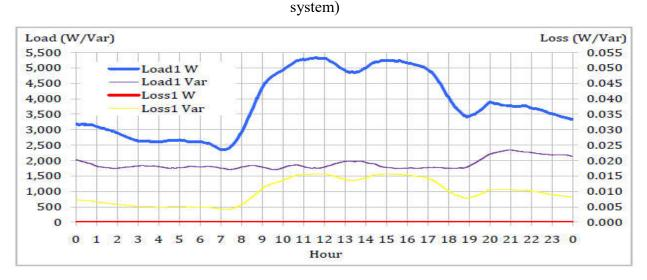
Fig.9. Total load and loss occur at sub-distribution system (tap position at optimal for 69-test bus system)
