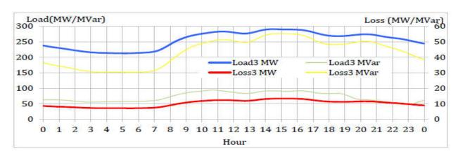
Fig.3.Total load and loss occur at transmission system (tap position at 1.0 p.u for 69-test bus
