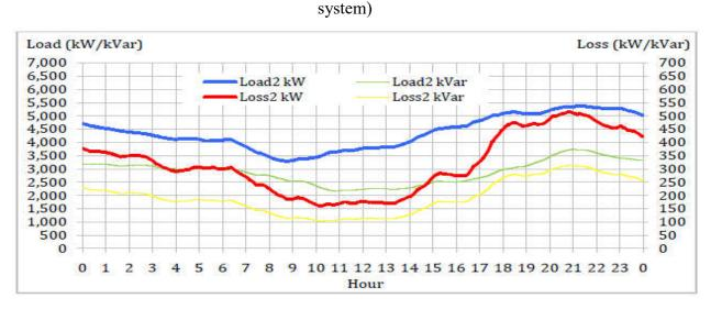
Fig.8. Total load and loss occur at distribution system (tap position at optimal for 69-test bus
