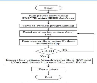
Fig.2. The simulation process for Phython programming
