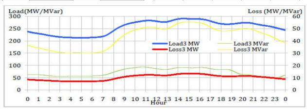
Fig.7. Total load and loss occur at transmission system (tap position at optimal for 69-test bus
