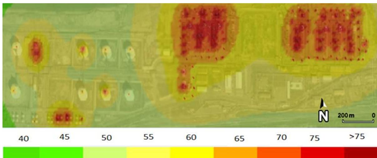
**Fig.10.**General noise mapping of the GP1Z plant
