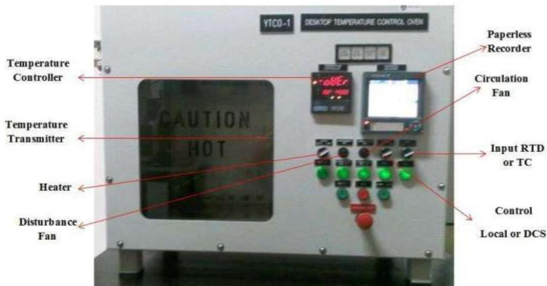
Fig.1. Temperature control plant [13]
