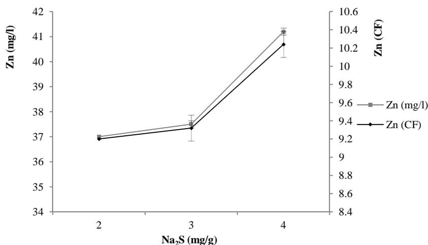
**Fig.9.** Na<sub>2</sub>S effect on Zn flotation at pH = 12 in rhmanolipids presence
