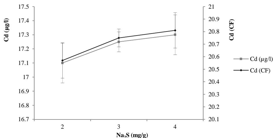
**Fig.10.** Na<sub>2</sub>S effect on Cd flotation at pH = 12 in rhmanolipids presence
