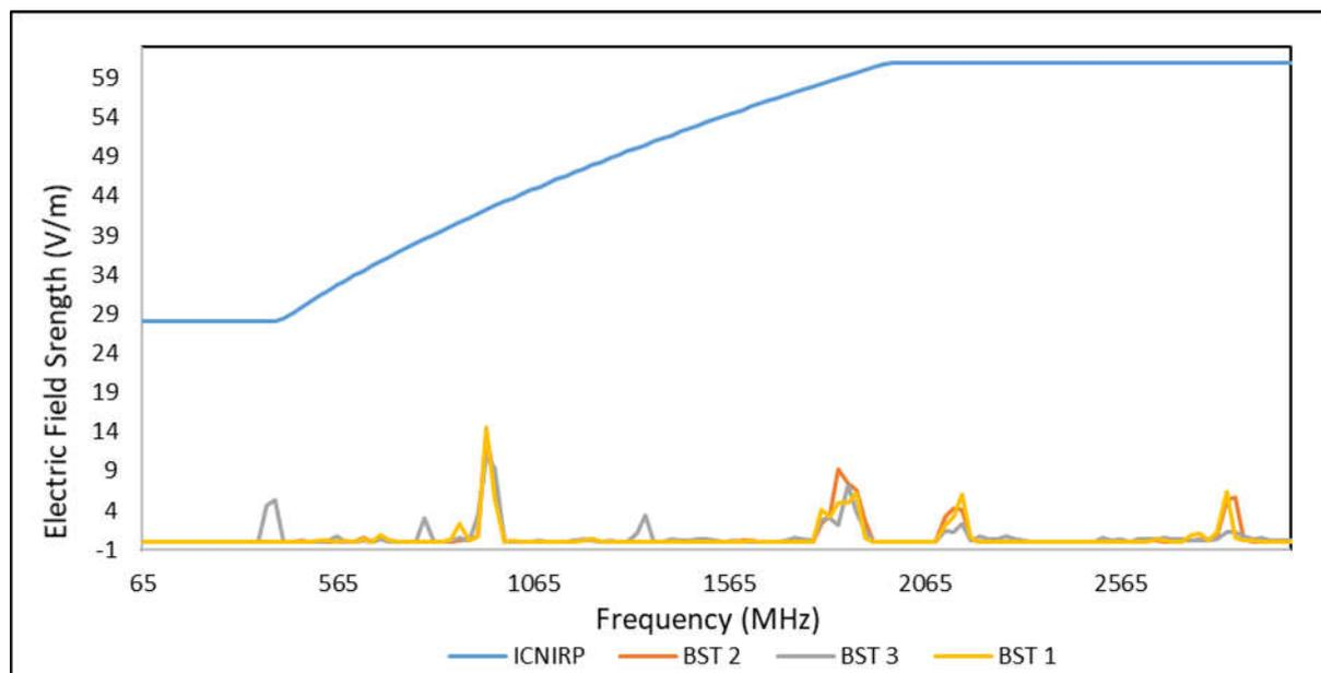
**Fig.5.** The comparison of EF strength with ICNIRP standard
