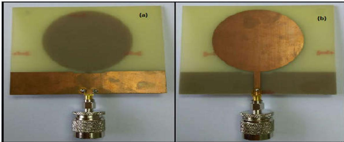
**Fig.2.** Circular patch antenna (a) rear view (b) front view
