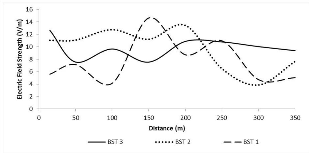
**Fig.4.** Trend of electric field strength measured at distances from BSTs
