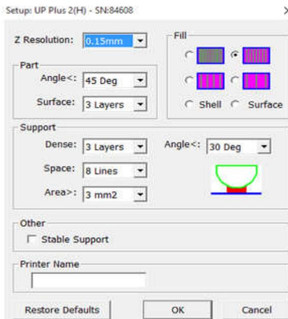
**Fig.2.** Print preference for FDM UP Plus 2 machine
