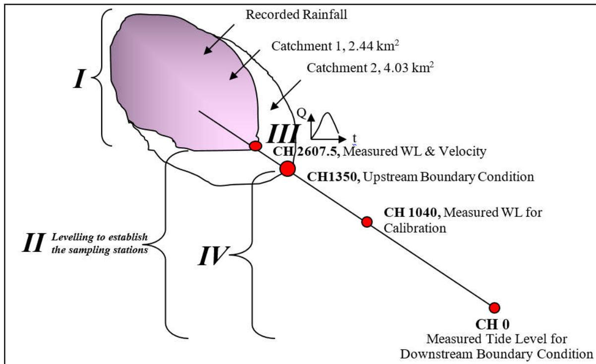
**Fig.5.** Sampling station for hydrologic and hydraulic model calibration and validation
