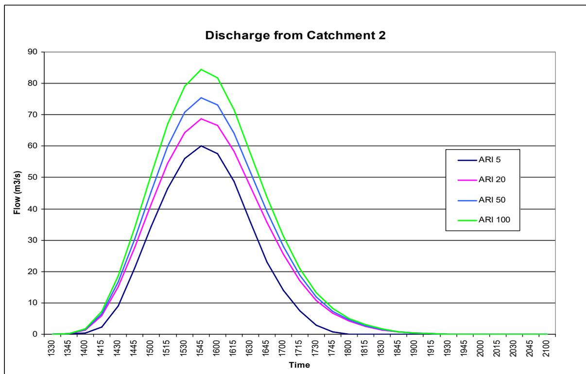
**Fig.10.** Discharges with 5 ARI, 20 ARI, 50 ARI and 100 ARI
