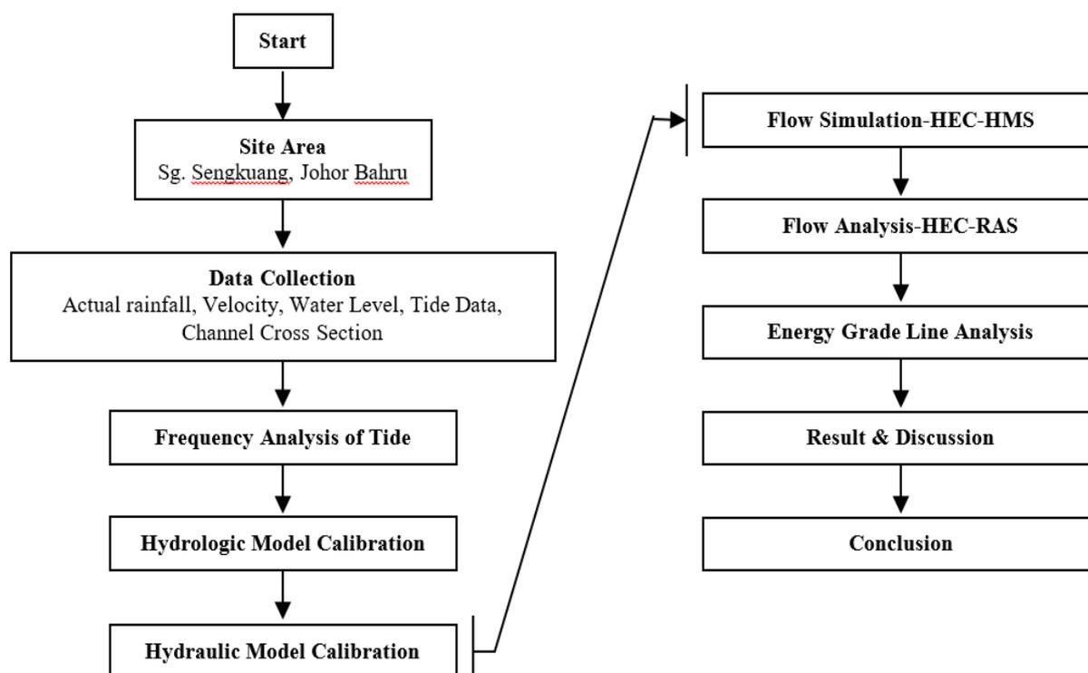
Fig.4. Hydrologic and hydraulic analysis of Sungai Sengkuang
