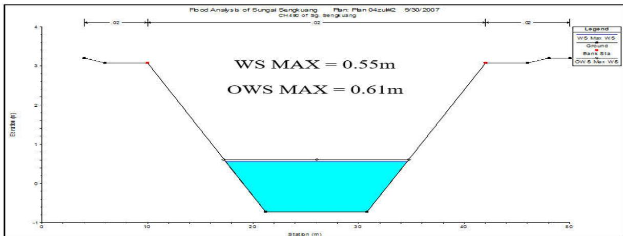
Fig.8. Calibrated water level at CH 1040
