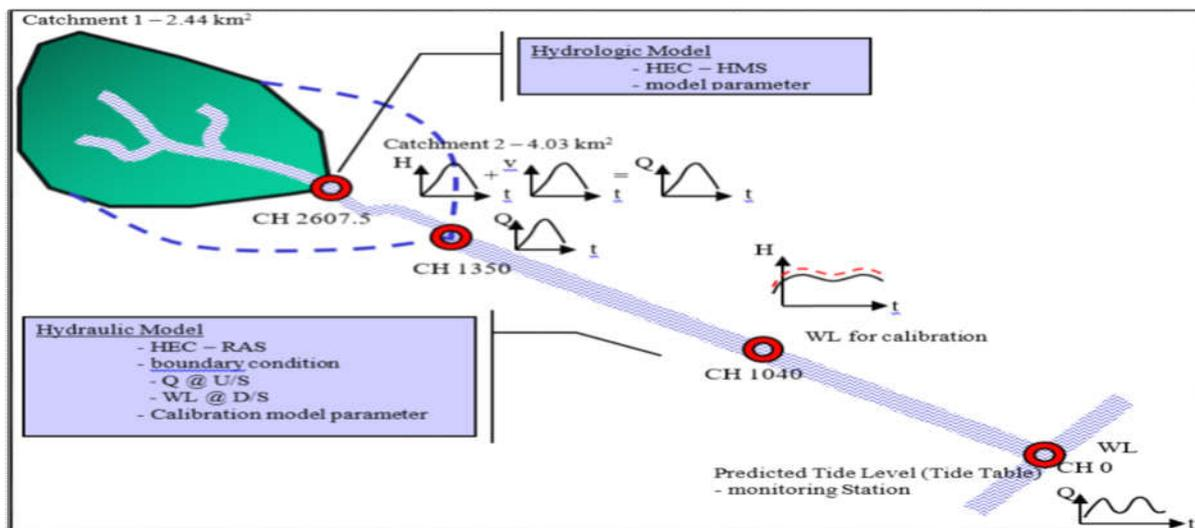
Fig.3. Schematization of hydrologic and hydraulic analysis
