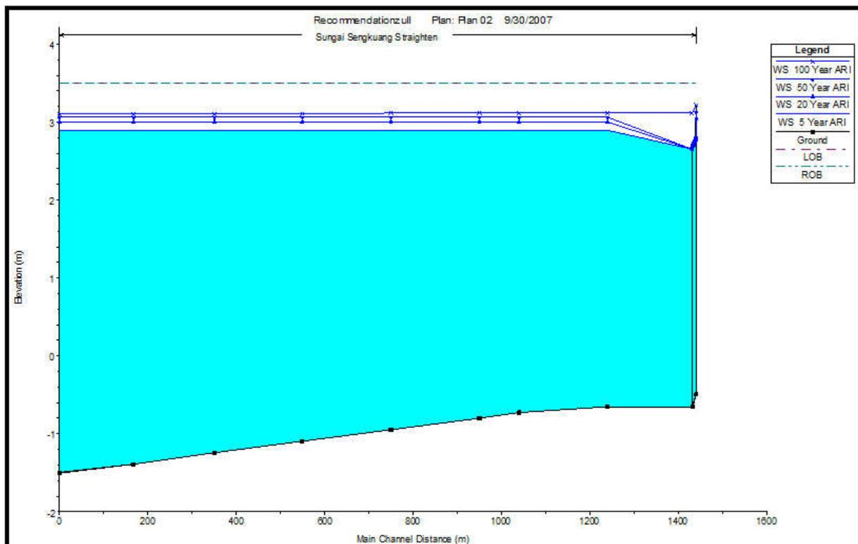
Fig.13. Water surface profile plot of proposed channel
