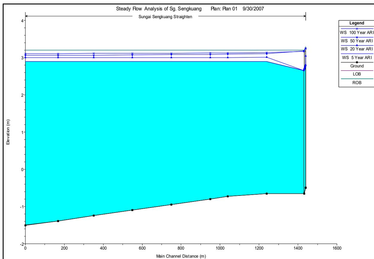
**Fig.11.** Water surface profile plot
