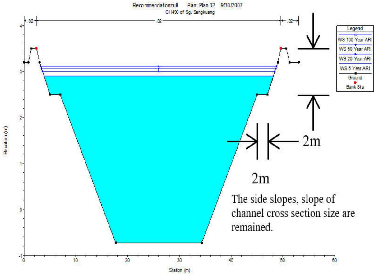
Fig.12. New cross section of proposed channel
