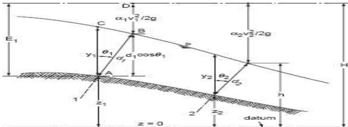
**Fig.1.** Open channel flow definition diagram
