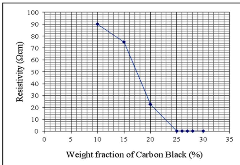
**Fig.2.** Resistivity of Nanocomposites with CB Filler loading.
