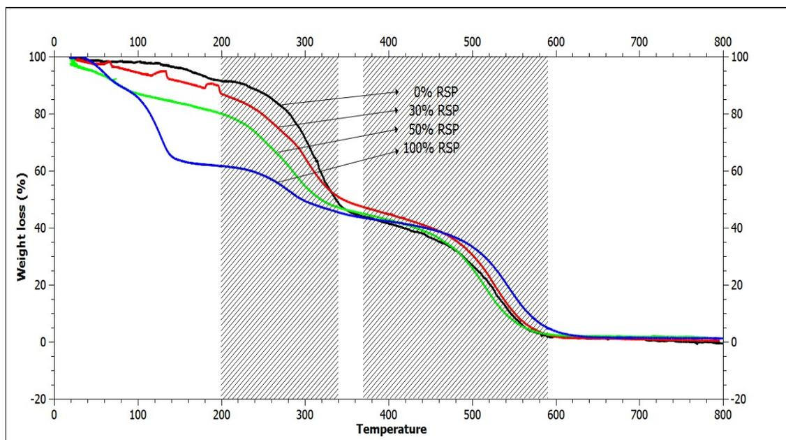
**Fig.4.** Thermo- gravimetric spectra of the polyurethane foams with varied amount of rice straw-based polyols (0%, 30%, 50% and 100%) replacement
