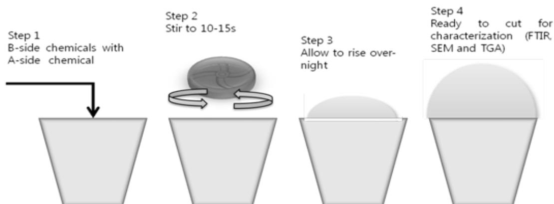
**Fig.1.** Procedure in synthesizing PU foam
