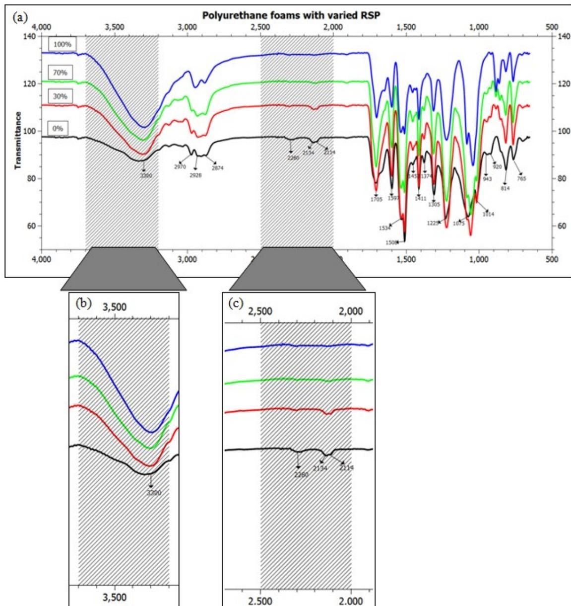
**Fig.3.** Over-all FTIR spectra of the PUF with varied amount of rice straw-based polyols (0%, 30%, 50% and 100%) replacement (b) in the region between 3100-3700  $\text{cm}^{-1}$  and between 2000-2500  $\text{cm}^{-1}$  (c).
