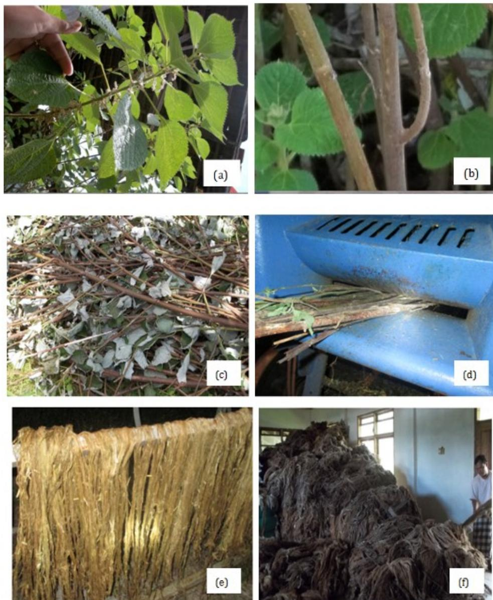
**Fig.1.** Processing of ramie plant to ramie fibers (a) ramie bloom (b) brown rod (c) rod and leaves (d) decortation (e) ramie fibers (f) china grass
