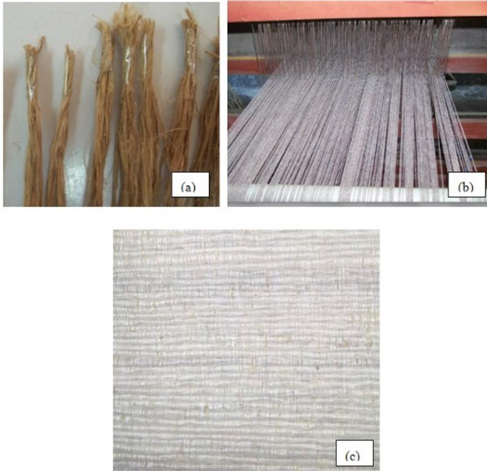
**Fig.2.** Processing ramie fibers to be composite reinforcement
