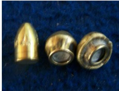
**Fig.7.** The projectile deformed
