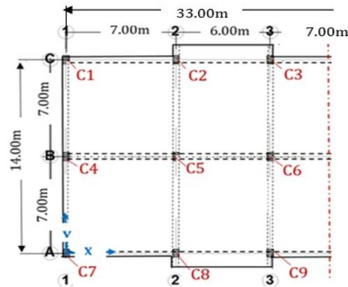
**Fig.2.** Choice of columns (C1- C9) to be studied on a given floor, considering the symmetry of their location on the horizontal plan
