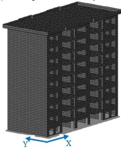
**Fig.5.** 3D finite element model (model 2) with masonry infill walls on all the stories
