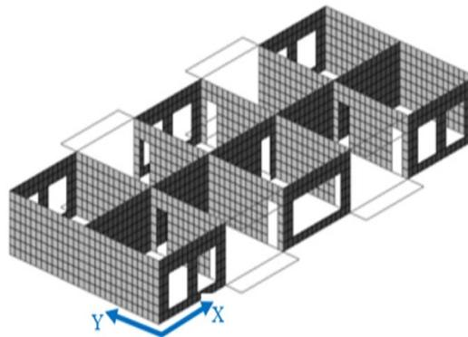
**Fig.3.** Location of the bearing masonry infill walls (with or without openings) on a floor
