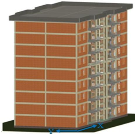
**Fig.1.** Architectural model of the studied nine-story cast-in-situ framed building
