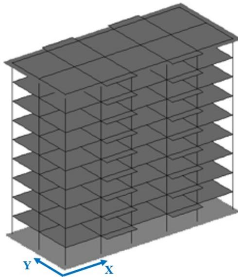
**Fig.4.** 3D finite element (model 1) of the studied cast-in-situ framed building without masonry infill walls
