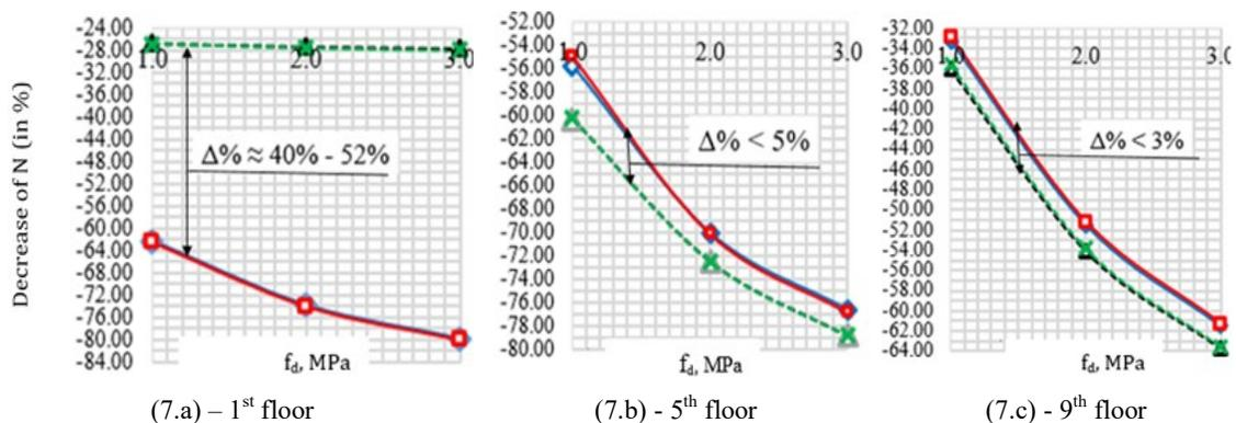
Fig.7. Decrease of longitudinal forces in internal columns according to the strength of the masonry infill walls and kind of loading: (a) on the lower floor; (b) on the middle floor; (c) on the upper floor
