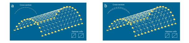
**Fig.3.** Finite-element 3D design model of a grid shell with square and rectangular cells: (a) without reinforcements and (b) with a diaphragm
