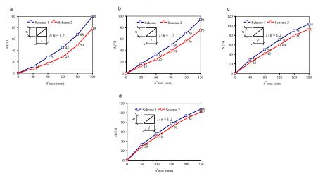
Fig.6. The effect of the introduction of joints with diaphragm elements on the percentage of depletion of the bearing capacity  $\Delta$  (%) and the maximum deflection  $\delta^{z}_{max}$  (mm) of single-layered cylindrical grid shells with rectangular mesh size: (a) 2.16×1.8 m, (b) 2.86×2.38 m, (c) 3.61×3.01 m, (d) 4.32×3.6 m
