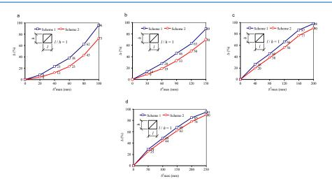
Fig.5. The effect of the introduction of joints with diaphragm elements on the percentage of depletion of the bearing capacity  $\Delta$  (%) and the maximum deflection  $\delta^{z}_{max}$  (mm) of single-layered cylindrical grid shells with square mesh size: (a) 1.8 m, (b) 2.38 m, (c) 3.01 m,
