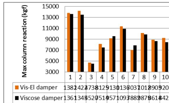
**Fig.8.** Comparison of peak response for collision of an intermediate and a steel moment frame for cases of viscoelastic and viscous dampers
