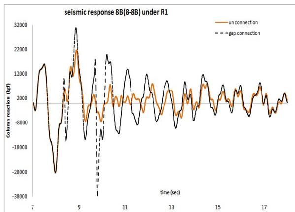
**Fig.3.** Free (-) and pounding-involved (--) Seismic response for collisions of an intermediate steel frame with a dual system of moment frame + invert bracing under record R1 of table 1.
