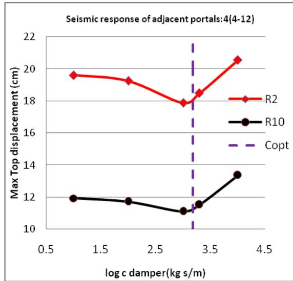
**Fig.5.** Peak response of two colliding intermediate steel frames for different records vs. damping of damper
