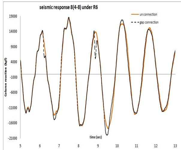
**Fig.4.** Free (-) and pounding-involved (--) Seismic response for collisions of two intermediate steel frames under record R6 in table 1
