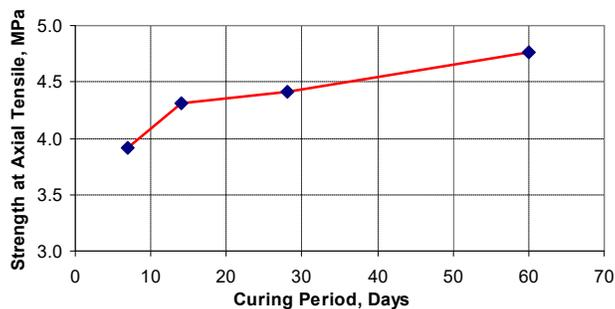
**Fig.4.** Dependency of the strength at axial tension on the curing period of HSCAC samples of 100x100x450 mm
