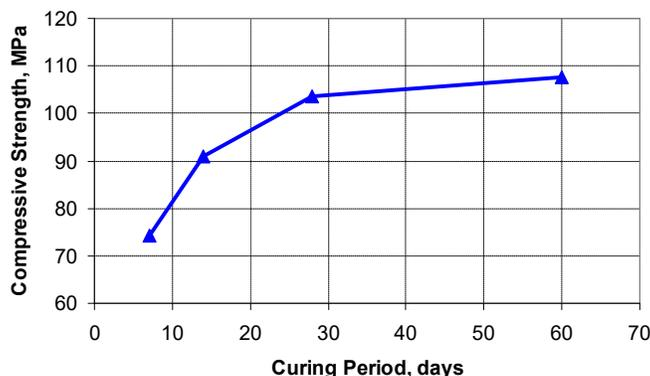
**Fig.1.** Compressive strength (cubic strength) of HSCAC depending on the curing period of HSCAC samples of 100x100x100 mm
