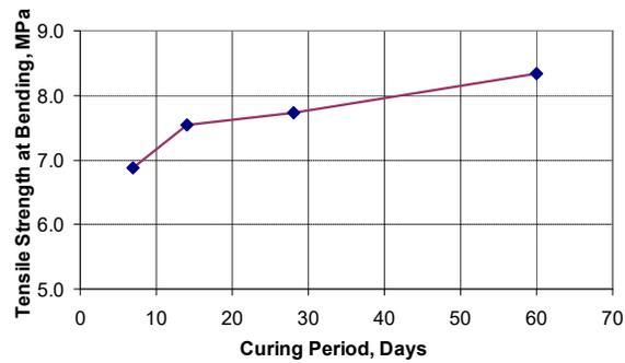
**Fig.3.** Dependency of the tensile strength at bending on the curing period of HSCAC samples of 100x100x450 mm
