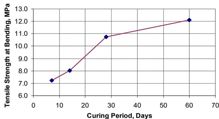
**Fig.3.** Dependency of the tensile strength at bending on the curing period of HSFPC samples of 100x100x400 mm
