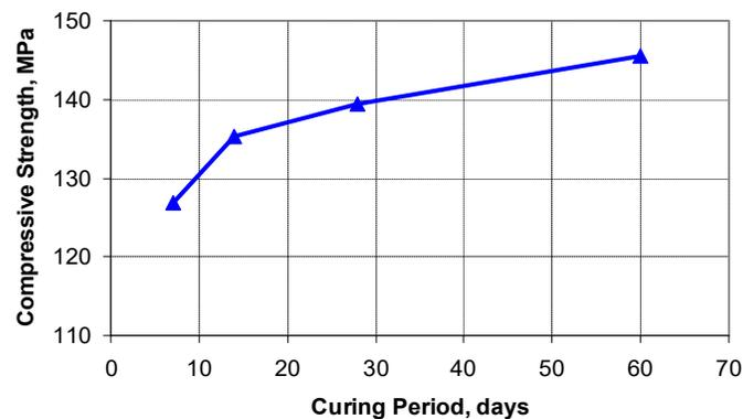
**Fig.1.** Compressive strength depending on the curing period of HSFPC samples of 100x100x100 mm
