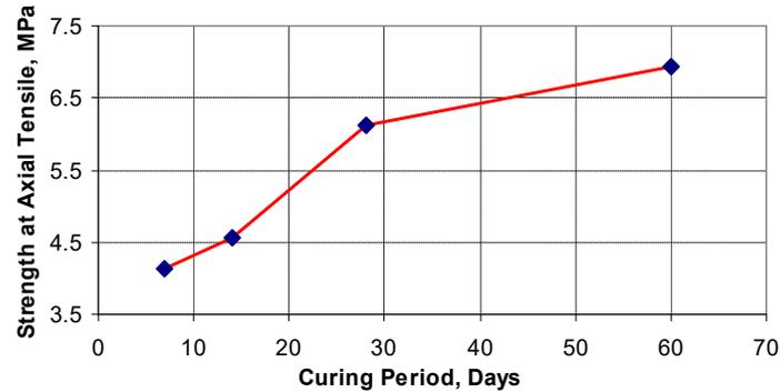
**Fig.4.** Dependency of the strength at axial tension on the curing period of HSFPC samples of 100x100x400 mm
