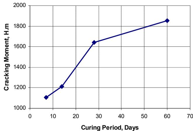
**Fig.2.** Dependency of the cracking moment on the curing period of HSFPC samples of 100x100x400 mm
