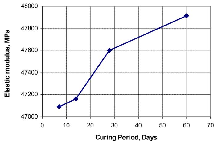
**Fig.5.** Dependency of the elastic modulus on the curing period of HSFPC samples of 100x100x400 mm
