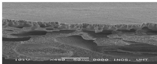
**Fig.3(a).** Cross section morphology of PV/TB 15-0 membrane
