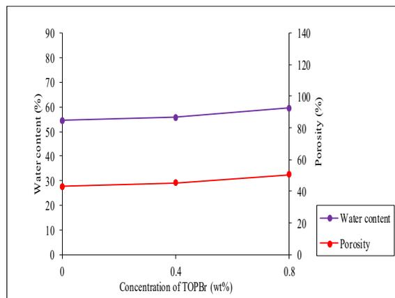
**Fig.1(b).** Water content and porosity at different concentration of TOPBr for PV/TB 17 membrane
