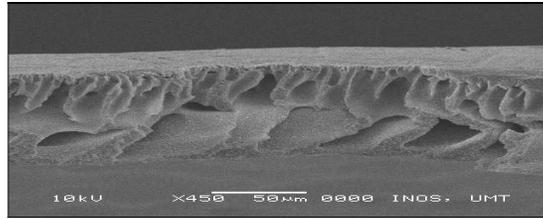
**Fig.3(b).** Cross section morphology of PV/TB 15-4 membrane
