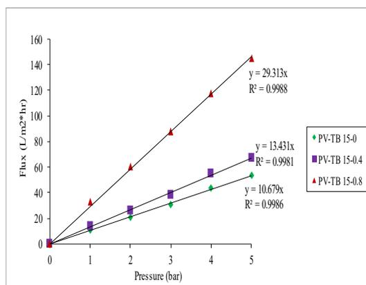
**Fig.2 (a).** Pure water flux of PV/TB 15 nanocomposite ultrafiltration membrane with different TOPBr composition
