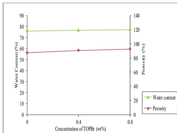
**Fig.1(a).** Water content and porosity at different concentration of TOPBr for PV/TB 15 membranes
