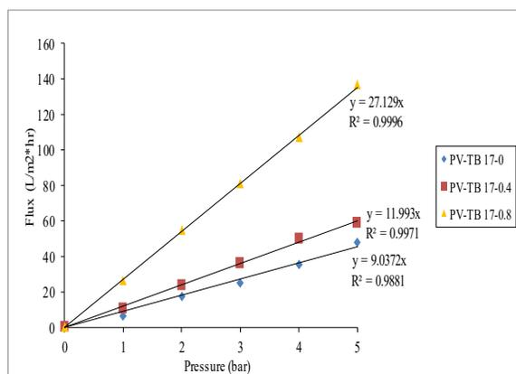
**Fig.2 (b).** Pure water flux of PV/TP-17 nanocomposite ultrafiltration membranes with different TOPBr composition.
