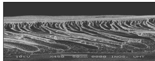
**Fig.4(b).** Cross section morphology of PV/TB 17-4 membrane
