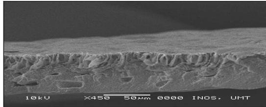
**Fig.3(c).** Cross section morphology of PV/TB 15-8 membrane
