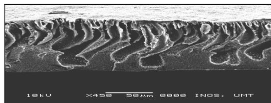
**Fig.4 (c).** Cross section morphology of PV/TB 17-8 membrane
