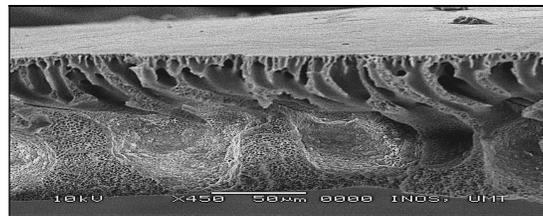
**Fig.4(a).** Cross section morphology of PV/TB 17-0 membrane
