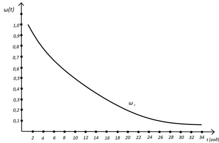
**Fig.3.** Dependence of quality parameters on time - welding joint ( $\omega_3$ )
