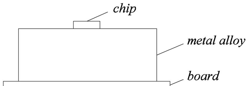
**Fig.2.** Simplified LED structure
