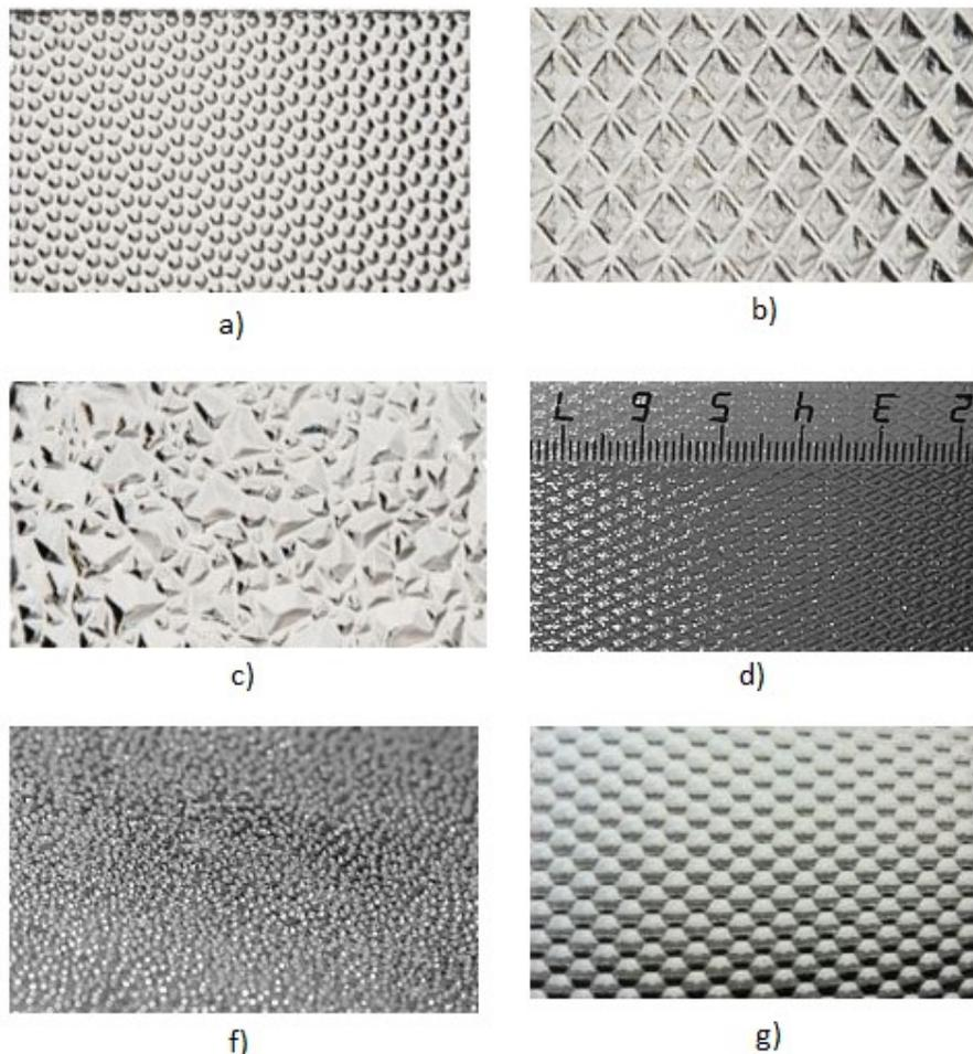
**Fig.1.** Diffusers for luminaires "Pin spot" (a), "Prism" (b), "Crushed ice" (c), "Microprism" (d), "Manka" (e), "Honeycomb" (f)
