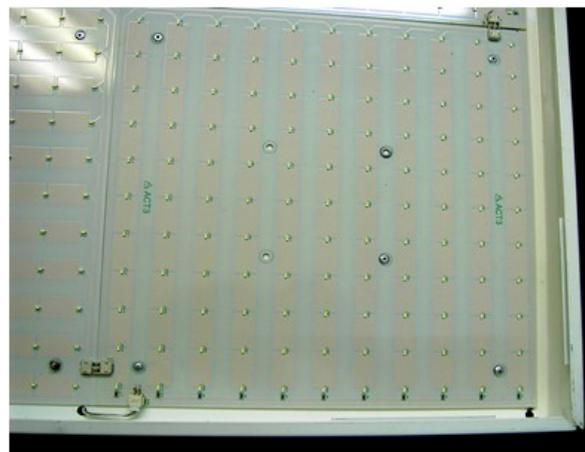
**Fig.4.** The location of 121 LEDs on  $\frac{1}{4}$  of the fixture area
