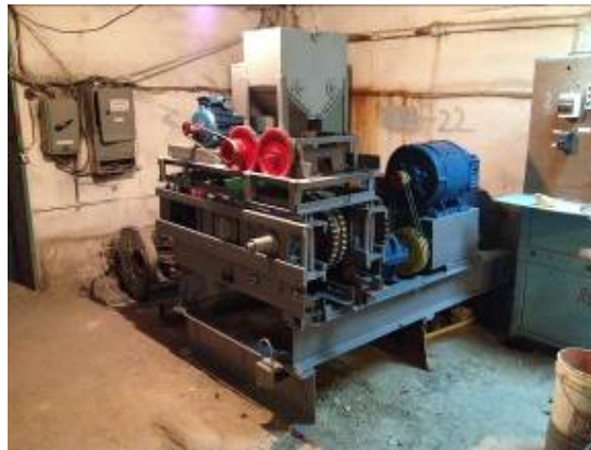
Fig. 5 Press rollers for man-made material briquetting:
