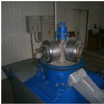
Fig. 7. Screw extruder (a) and press roller extruder with a flat matrix (b)
