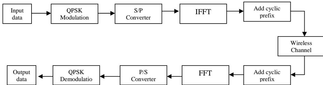
**Fig.1.** Diagram block conventional OFDM transceiver
