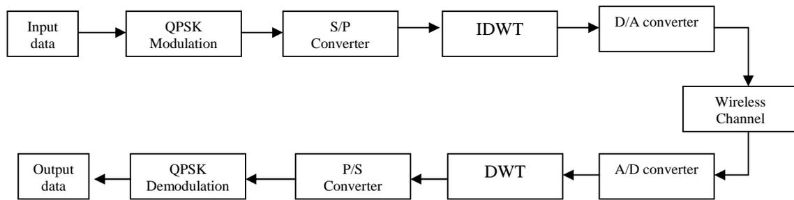
**Fig.2.** Block Diagram of Wavelet OFDM
