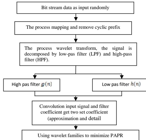
**Fig. 3.** The flow chart Wavelet based OFDM
