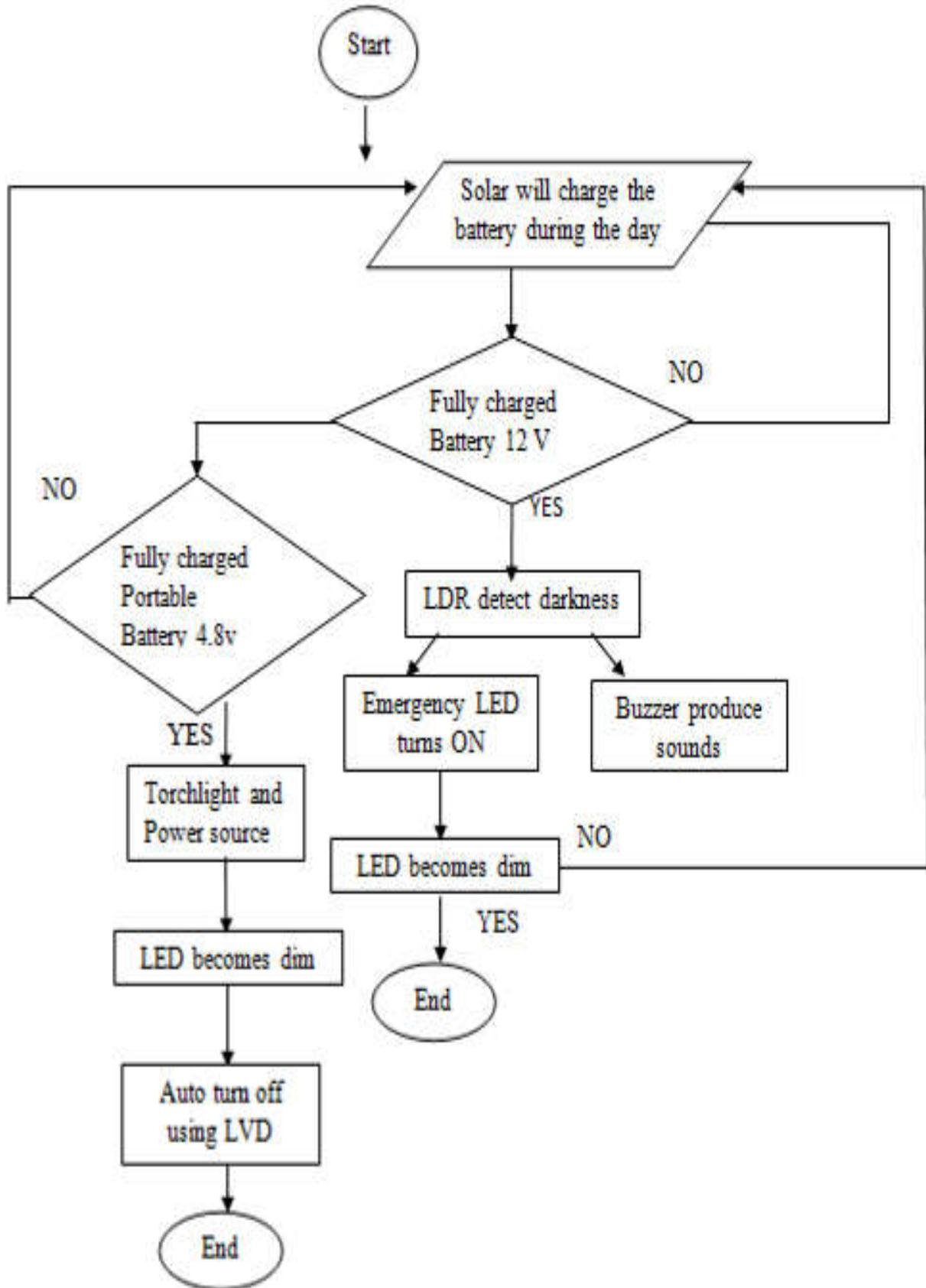
Fig.4. Flow chart of smart portable solar light
