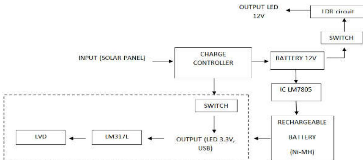
**Fig.1.** Circuit operation of smart portable solar light
