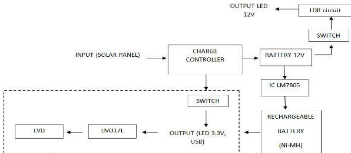
**Fig.1.** Circuit operation of smart portable solar light
