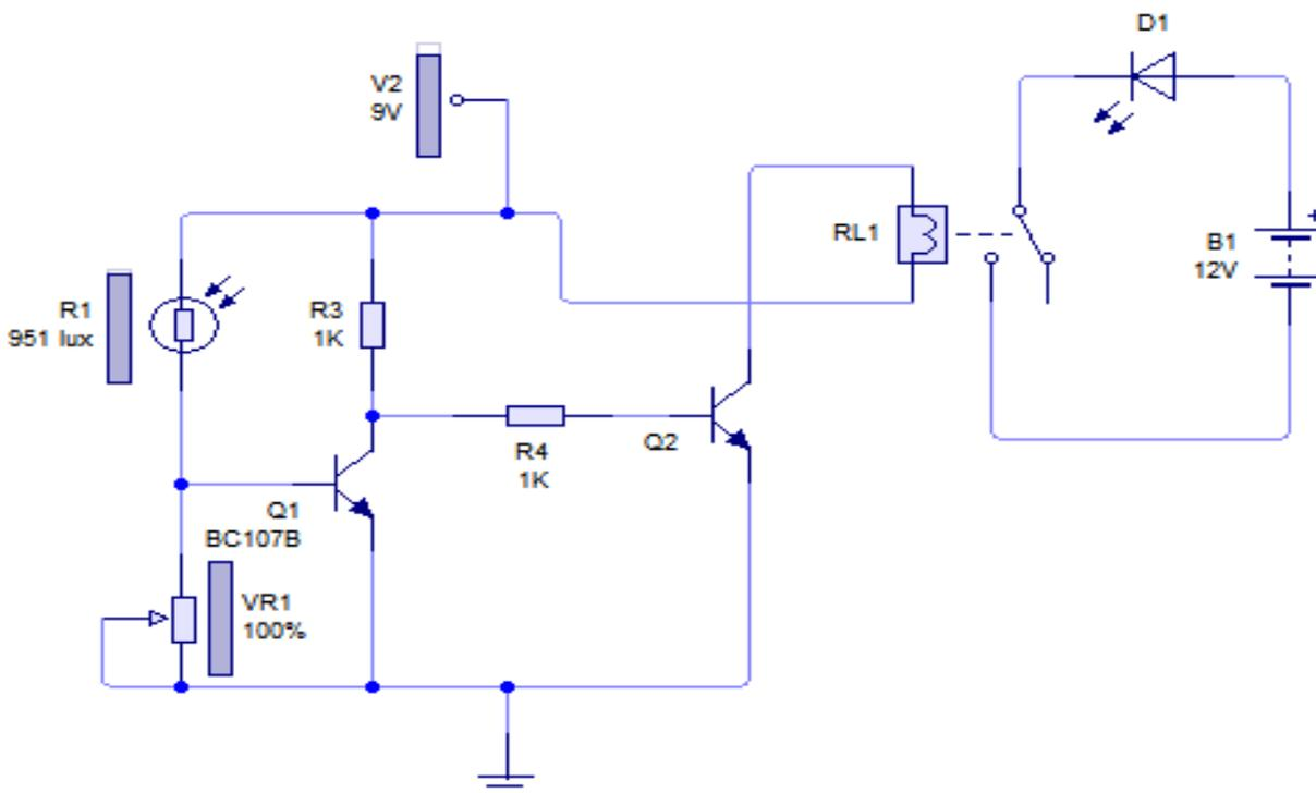
Fig.3. Emergency LED circuit
