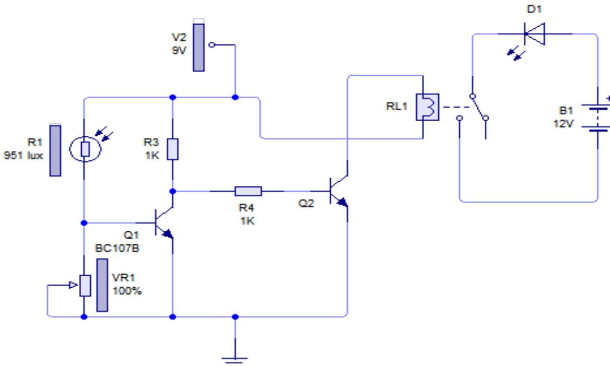
Fig.3. Emergency LED circuit
