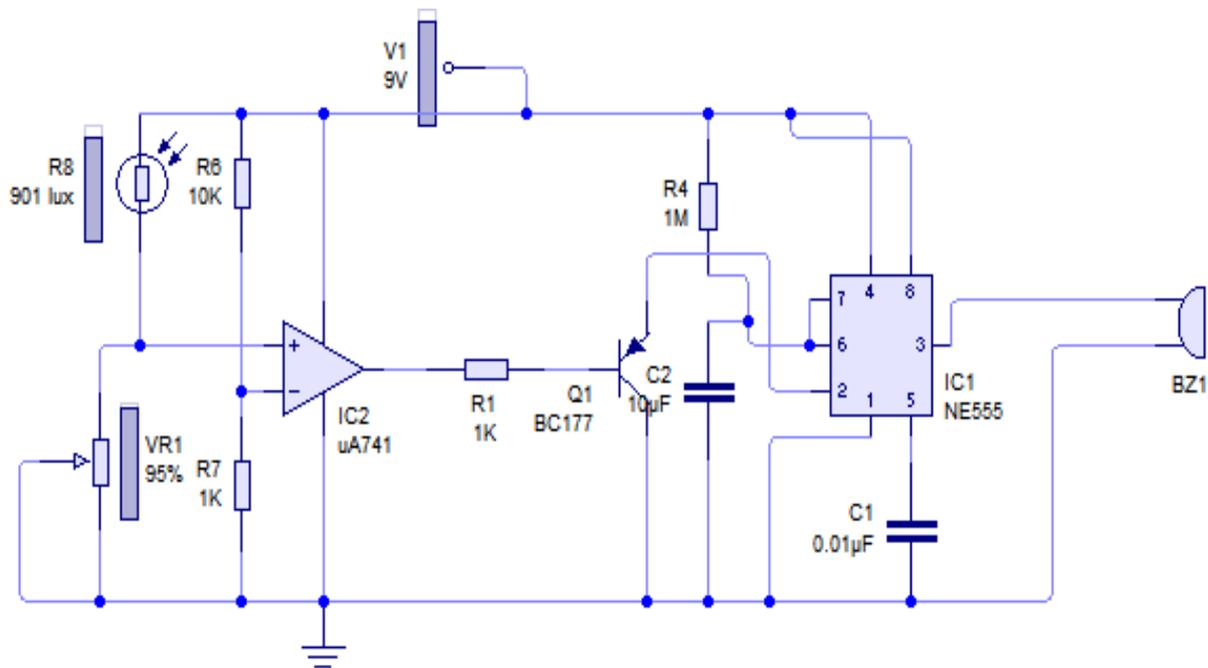
Fig.2. Emergency alarm circuit
